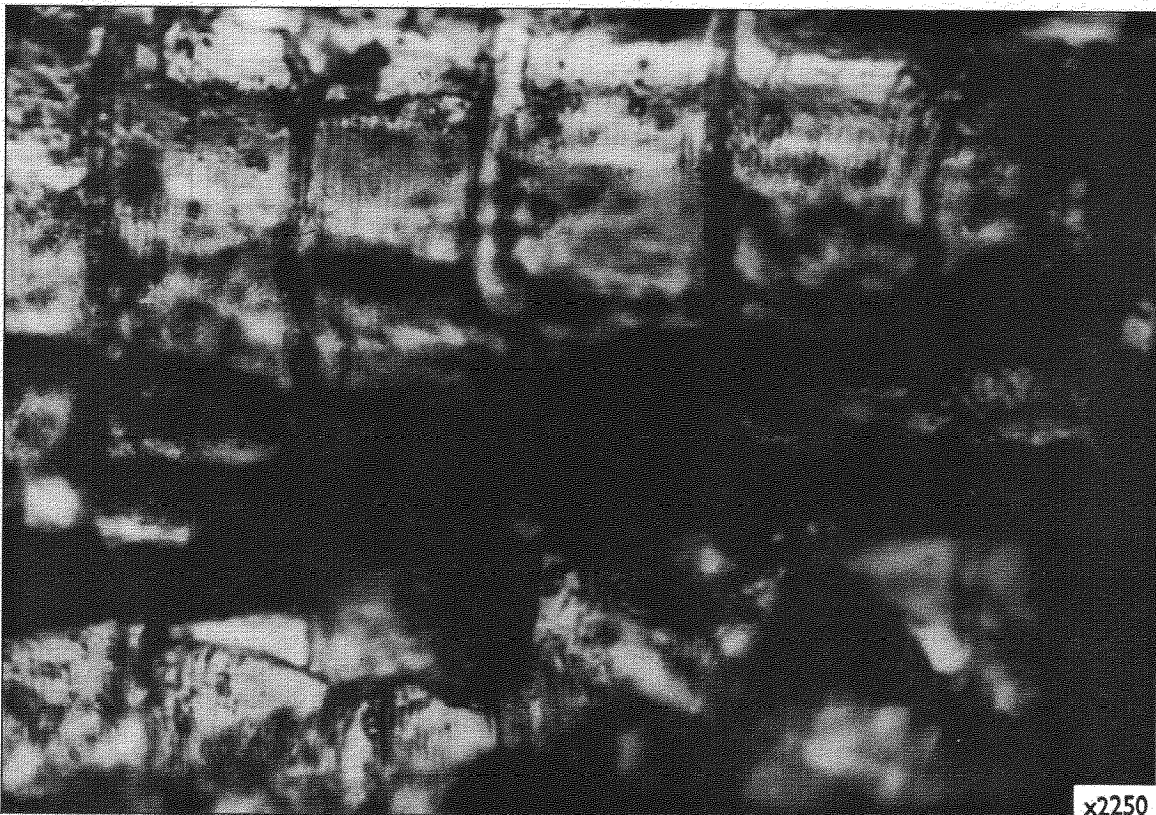
FIG.25. STRIATIONS FROM INDIVIDUAL GUST LOAD CYCLES
