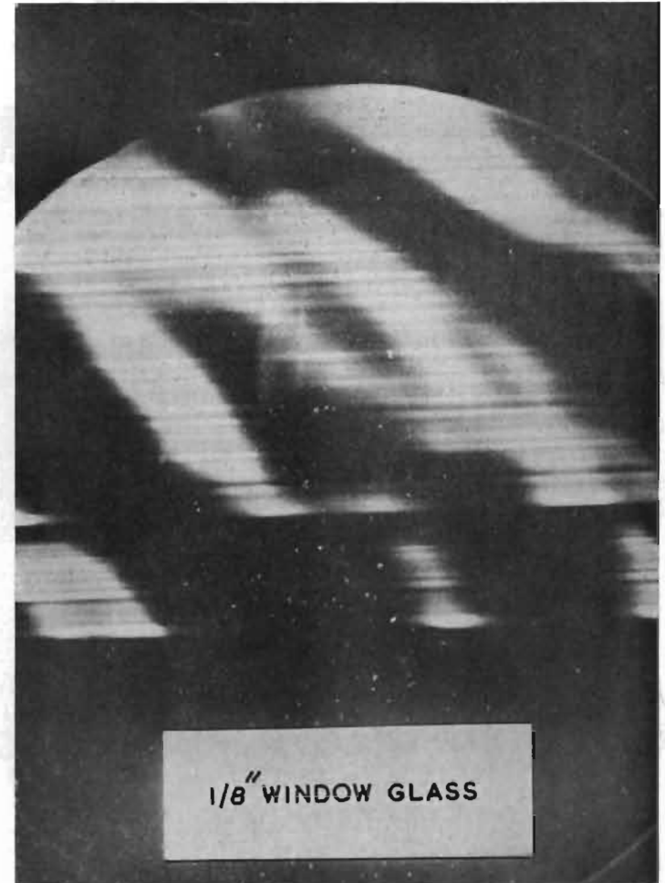
(b) Schlieren photograph of \frac{1}{8} -in. sheet of window glass, showing surface waves.
