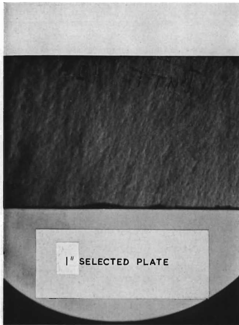
FIG. 69. Schlieren photographs of 1 in. sheet of selected plate glass showing wedge-shaped nature.
