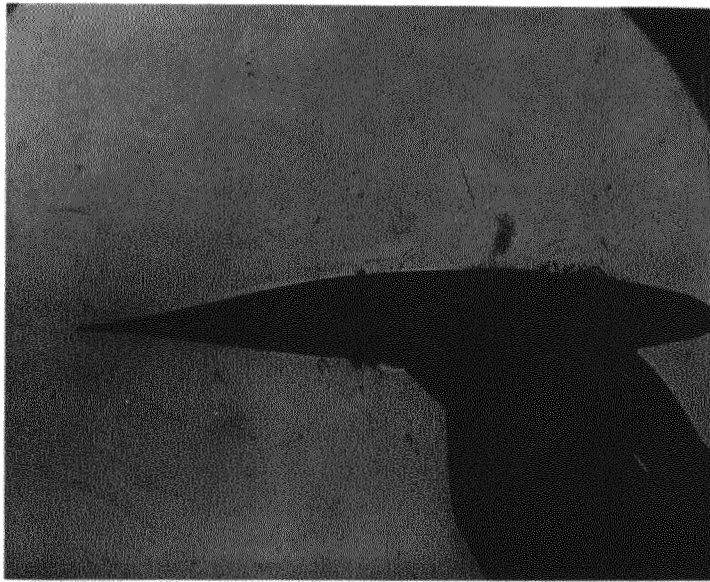
FIG. 3. Aerofoil G 1442/1547 at \alpha = 0.5 deg. Control photograph at zero Mach number.
