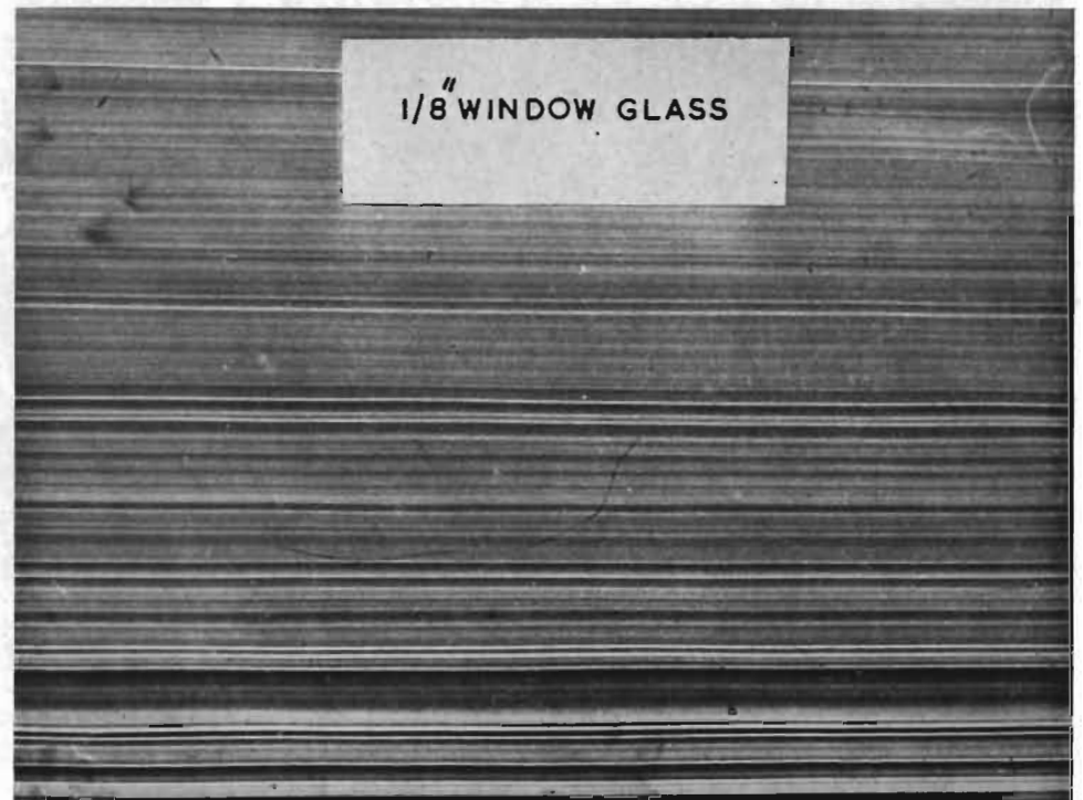
Direct-shadow photograph of \frac{1}{8} -in. sheet of window glass.
