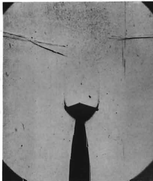
FIG. 88. Photograph showing wake and shock-waves behind an aerofoil with brake flaps. (Combination G.) M = 0.78 .
