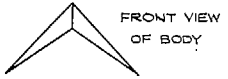
(c) CARET BODY WITH CONSTANT ANHEDRAL (I.e. A TRIANGULAR CAPTURE FLOW TUBE).
