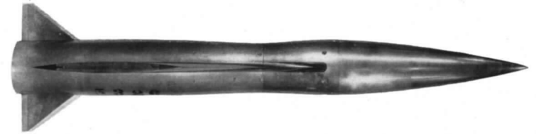
b. AREA RULE FOR M = 1.41 . MODEL No.75
