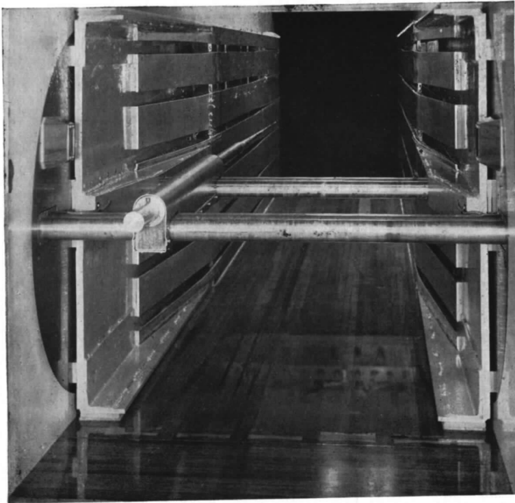
FIG. 5a. The liners as first tested, with the slats continued through the extraction region (with the cross shafts and calibrating probe).
