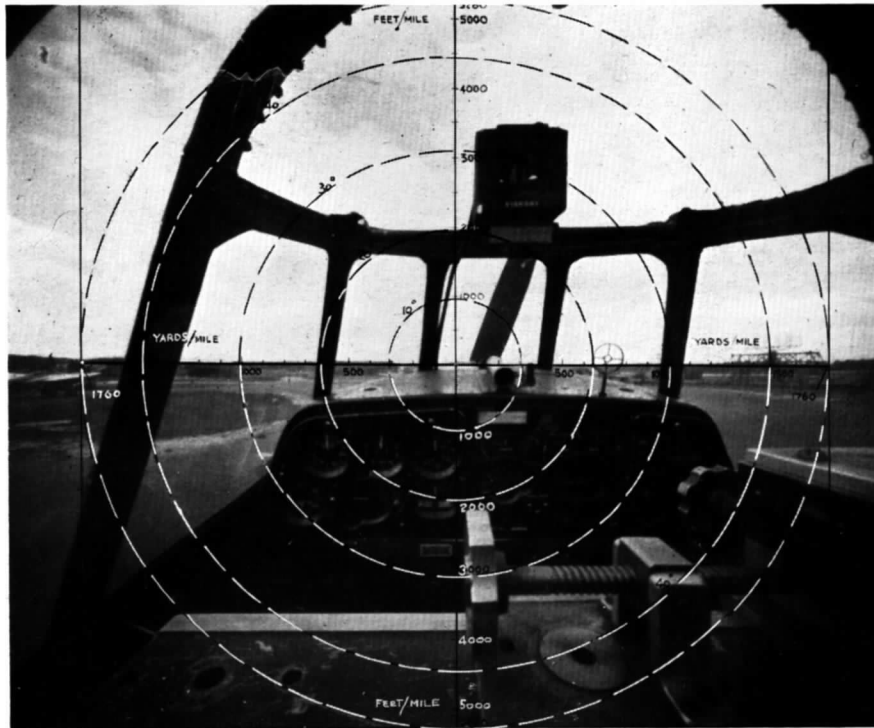
Photograph A. Camera position corresponding to pilot's left eye when seated with head central, seat fully up. Centre of graticule corresponds to a direction of sight inclined down at 13.3^\circ to wing chord.
