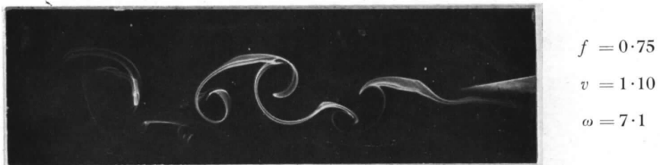
FIG. 10. Flow position at low frequency and wind speed. Nozzle at position 2.
