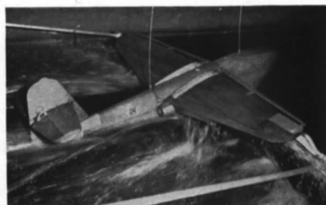
FIG. 24. Take-off at overload 17,250 lb. Seaworthiness tests.
