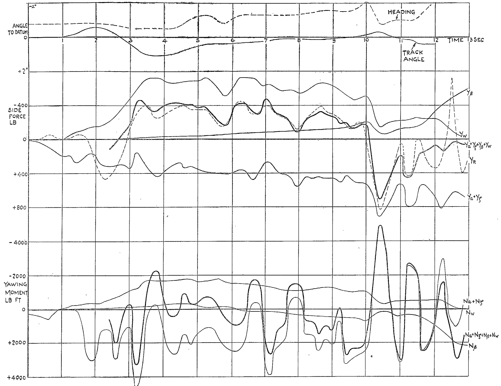
FIG. 14. Side-force and yawing-moment analyses. Flaps 0 deg.
