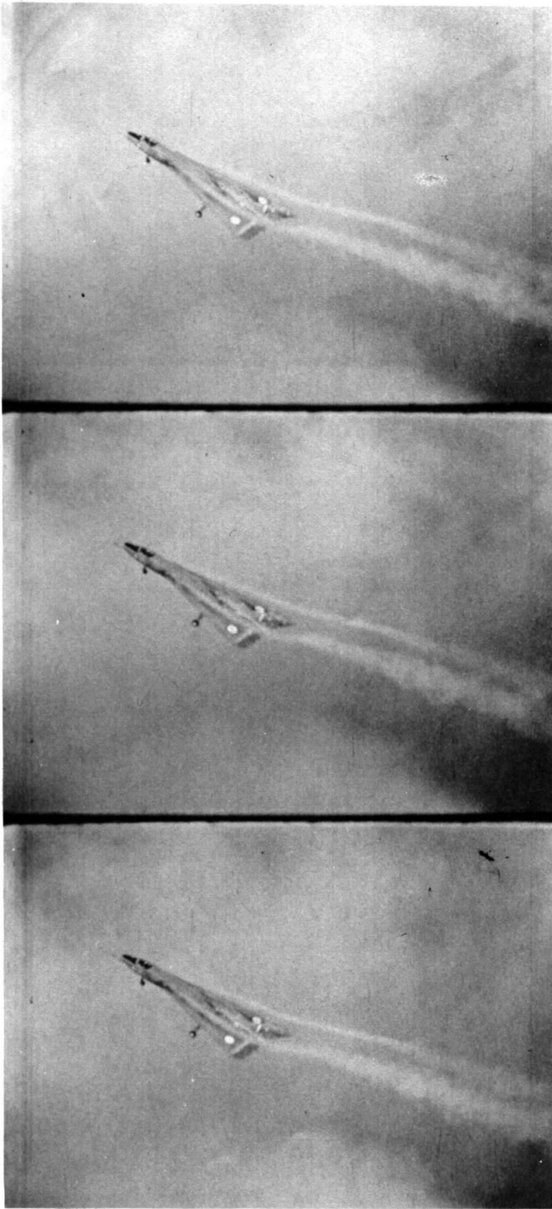
FIG. 6. Vortex breakdown at 30^\circ incidence while sideslipping to port (extract from cine film).
