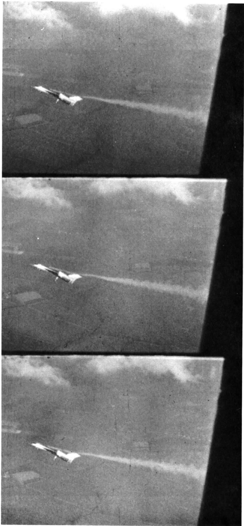
FIG. 5. Vortex breakdown at 28^\circ incidence (extract from cine film).
