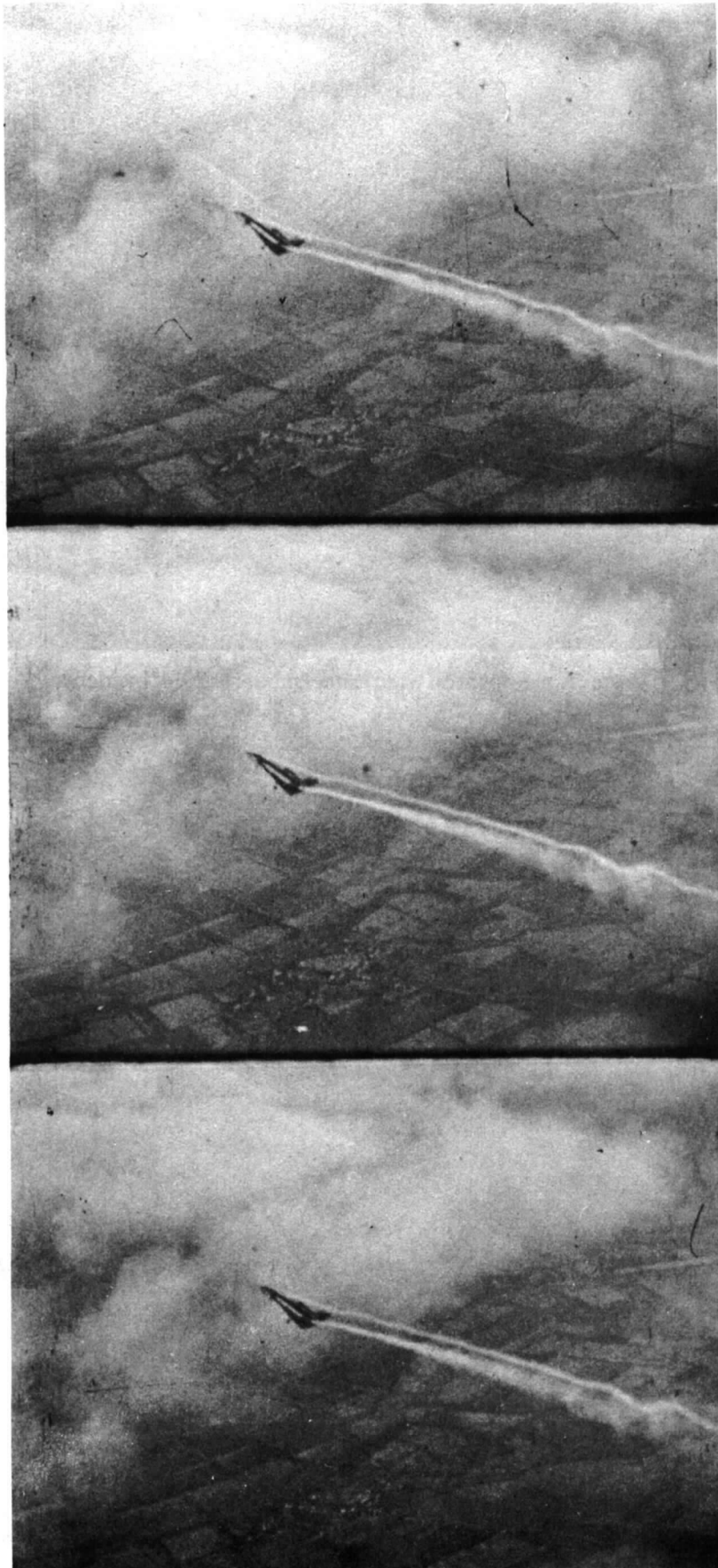
FIG 8. Vortex breakdown at 26° incidence while sideslipping to port.
