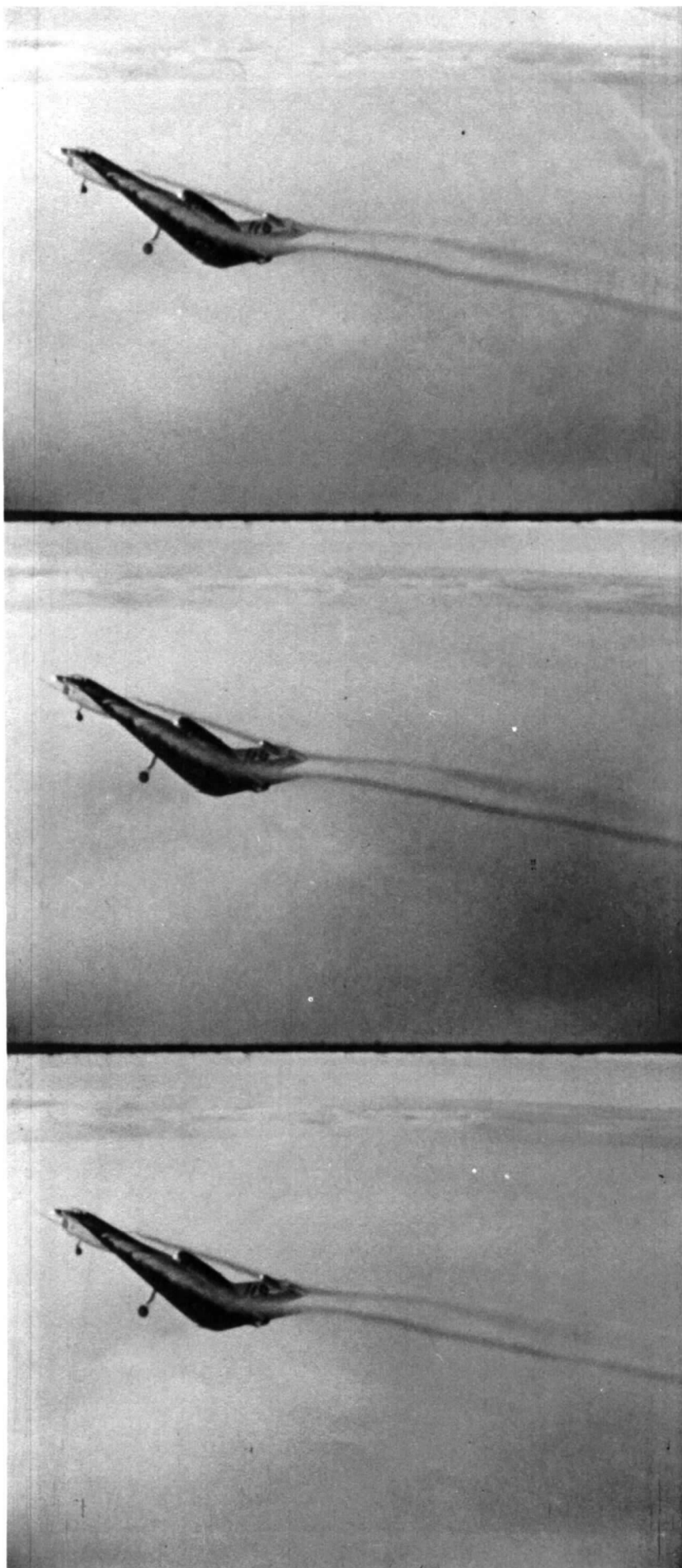
FIG. 7. Vortex breakdown at 28^\circ incidence while sideslipping to starboard.
