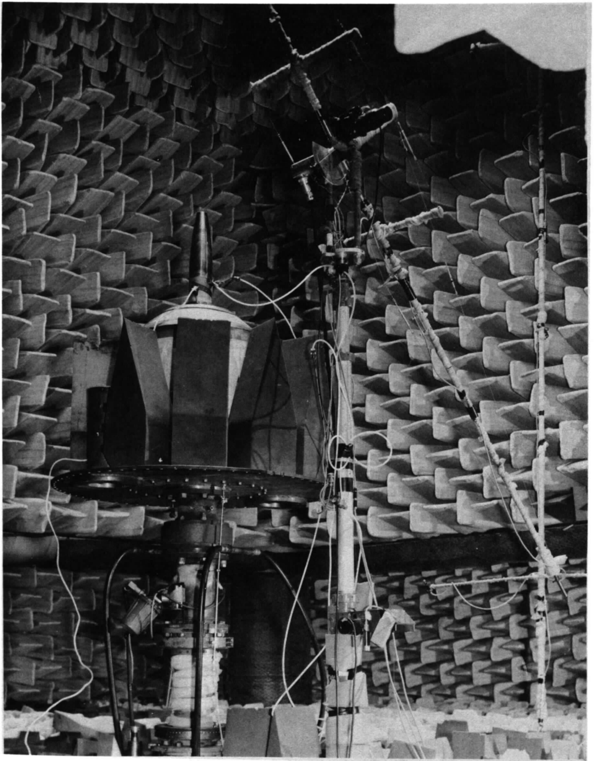
FIG. 4. Jet rig in anechoic chamber.
