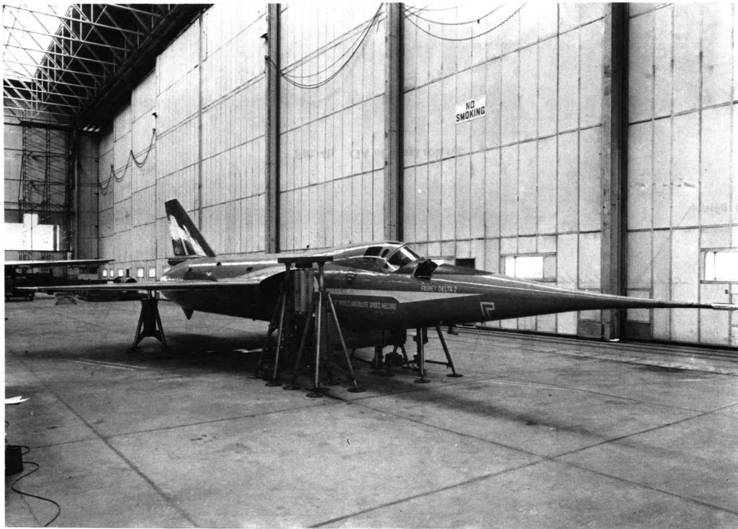
FIG. 5a. Aircraft on pitching moment of inertia rig.
