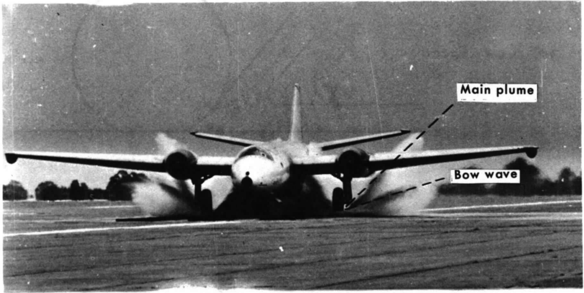
(a) Bow wave and main plume at V/\sqrt{P} \doteq 9
