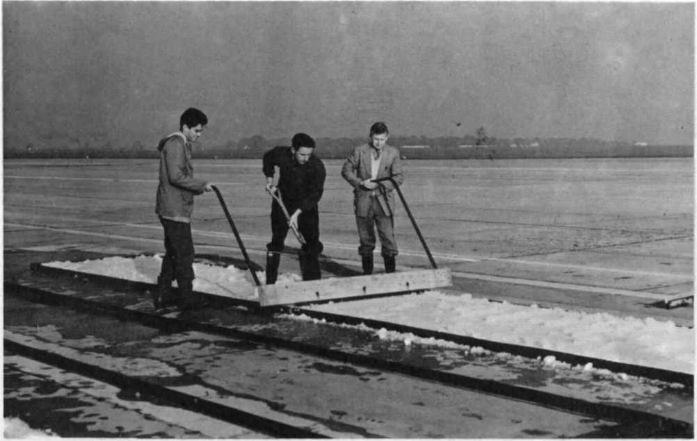
FIG. 6. Scraper and ice in ponds. The scraper runs on knife edge wheels and the blade height is adjustable.
