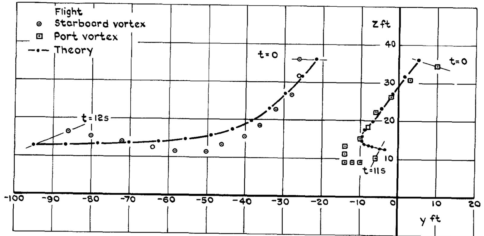
Fig.6 Comparison of measured and theoretical vortex positions
