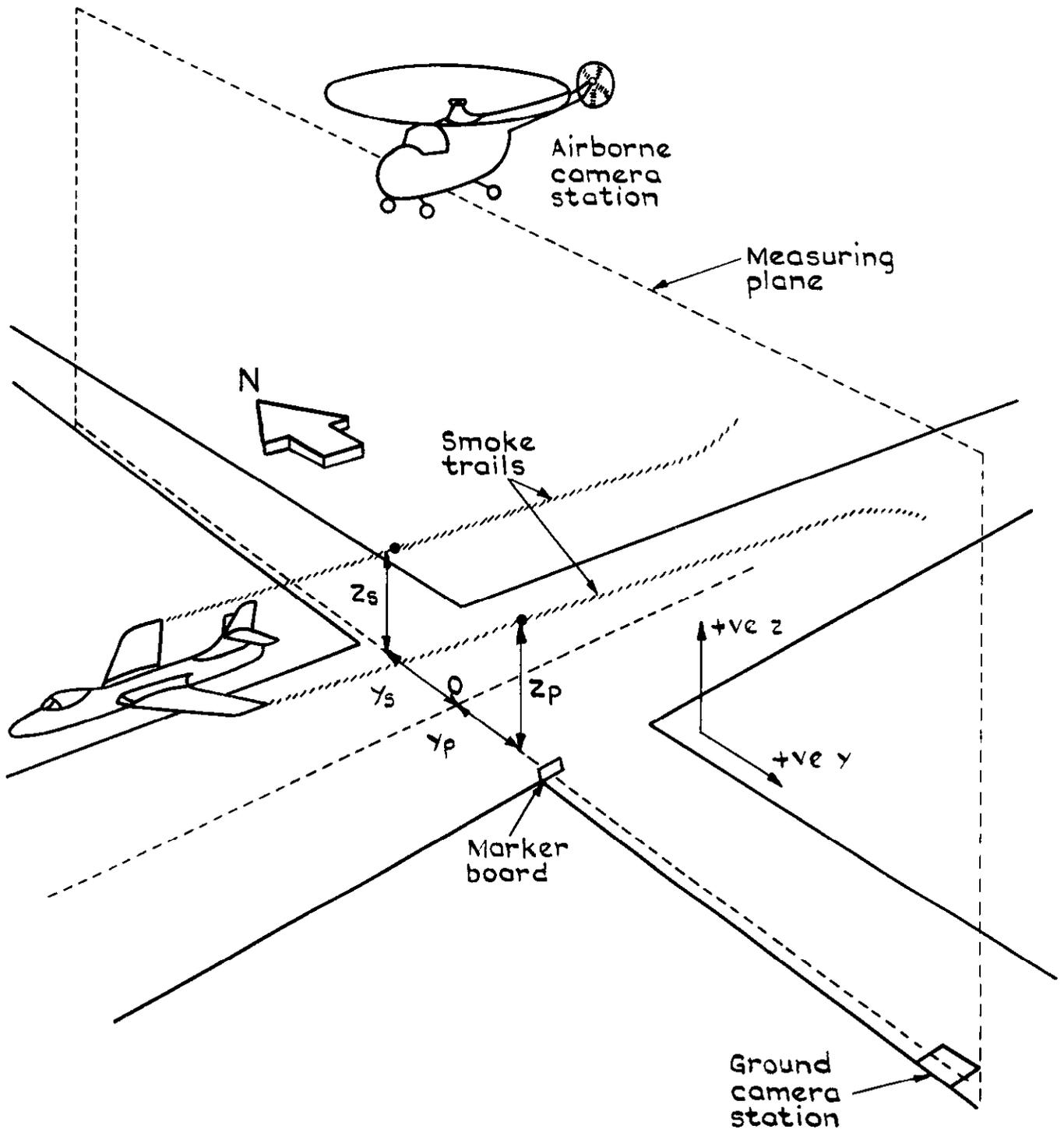
Fig.1 Diagrammatic view of test area
