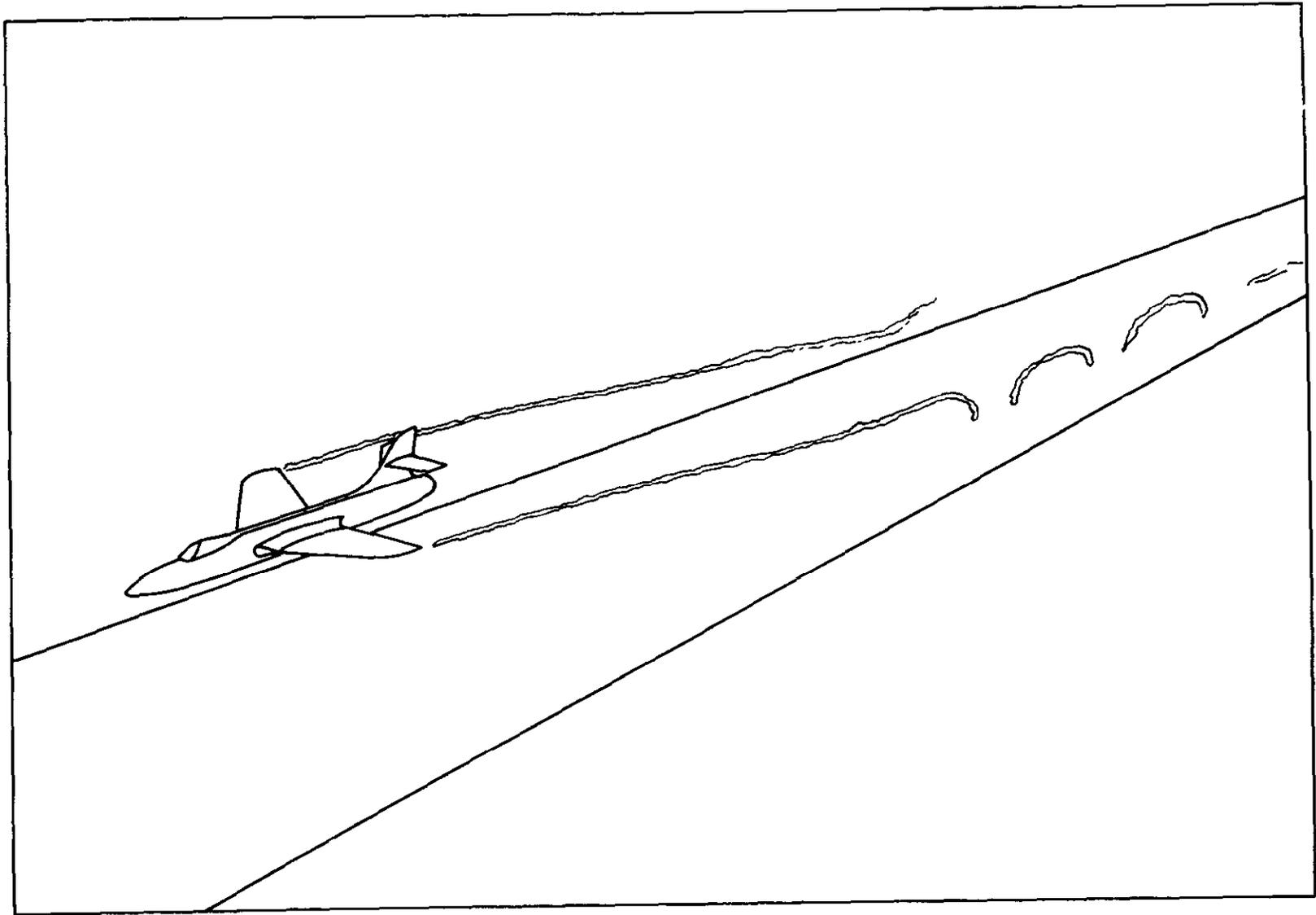
Fig 3 Sketch showing interaction sometimes observed between individual vortices and the ground
