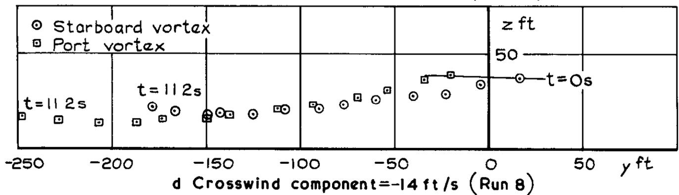
Fig 4a-d Measured vortex positions with different crosswind components
