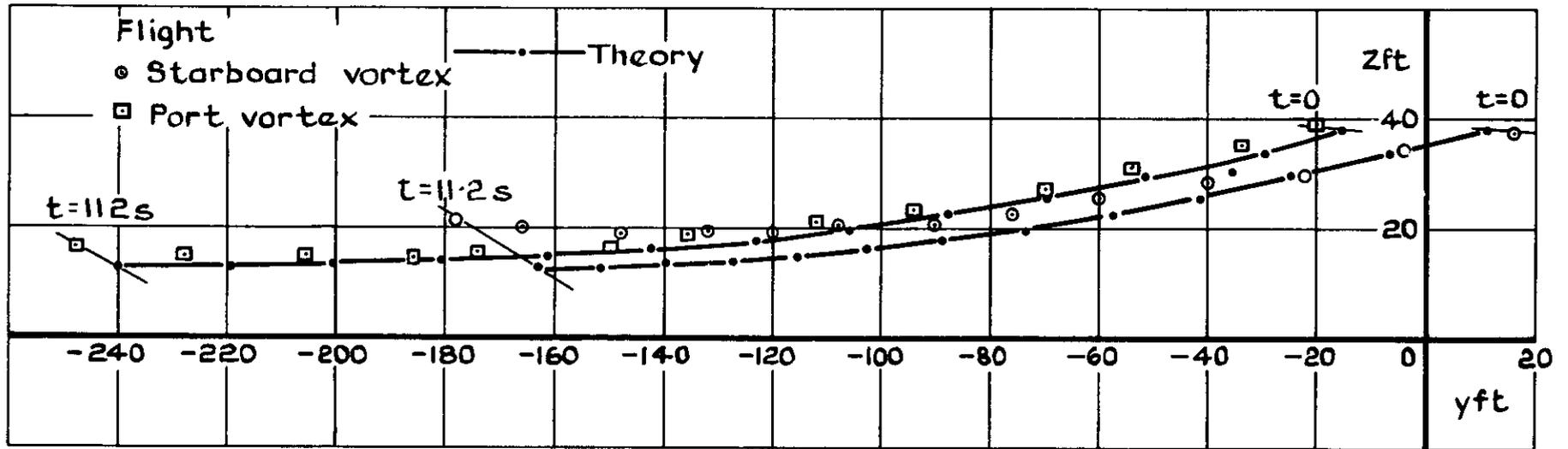
Fig. 8 Comparison of measured and theoretical vortex positions
